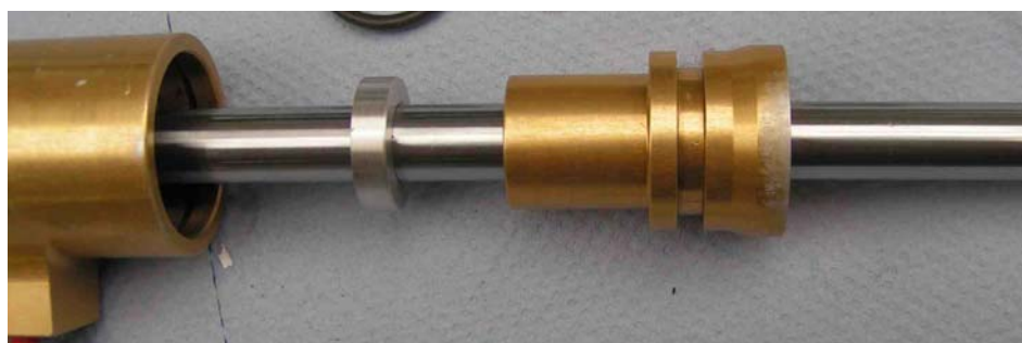
Fig. 6: Installed spacer bushing
