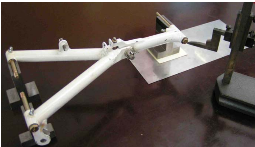
Fig. 3: Testing of radius strut adjusting (for example)
