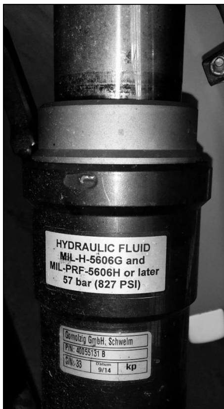
Figure 6.1: Present Fluid Pressure Placard and Serial Number Placard on shock absorber
